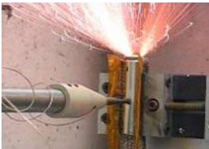
Figure 3-7: Internal Short Caused by Nail Penetration of a \text{LiCoO}_2/\text{Graphite} Cell at 4.2 V [20]
