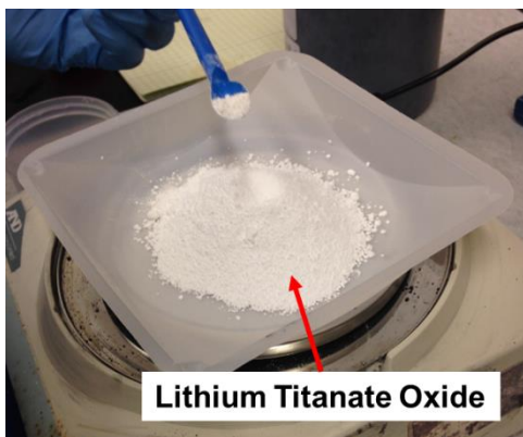
Figure C-4: Weighing Lithium Titanate Oxide Particles Prior to Inserting into Slurry Mixing Jar
