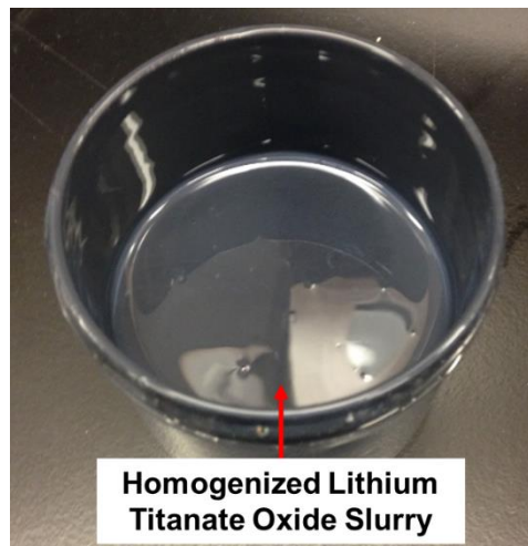
Figure C-6: Homogenized LTO Slurry; Ready for Electrode Coating
