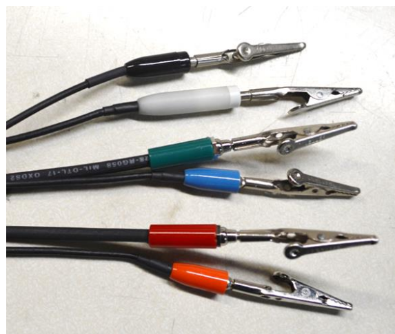
Figure 4-12: Gamry Reference 300 Potentiostat Leads
