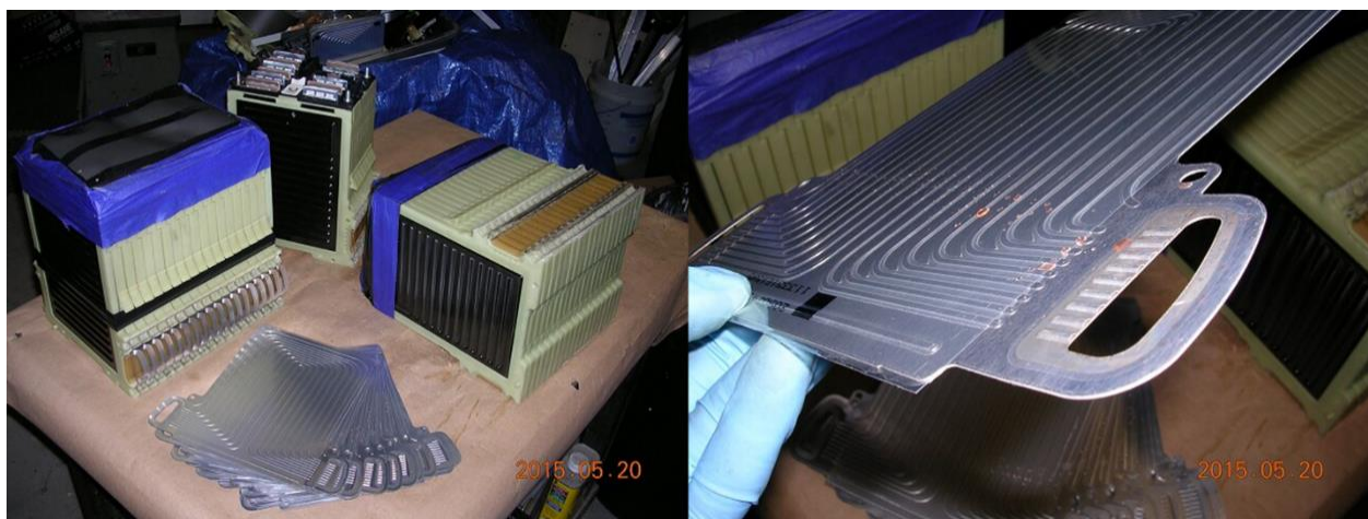
Figure 2-8: Aluminum Cooling Plates Used in Chevrolet Volt Battery Pack [63]
