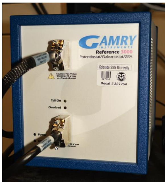
Figure 4-8: Gamry Reference 3000 Potentiostat
