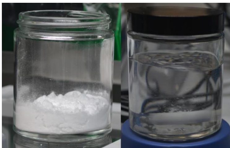
Figure 4-3: Unsolvated LiTFSI Salt (Left) and MFE Solution (1 M LiTFSI in 1:1 HFE-7000/EMC by Volume) on Stir Plate (Right)
