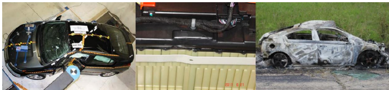
Figure 1-10: Chevrolet Volt Event Series (Left: Side-Impact Test, Middle: LIB Pack Damage, Right: Post Thermal Runaway Event) [38]
