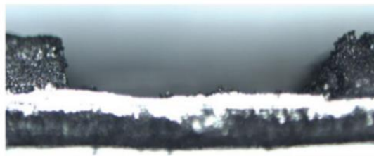
Figure 3-4: Representative Vapor Generation Channel Created in a Positive Electrode
