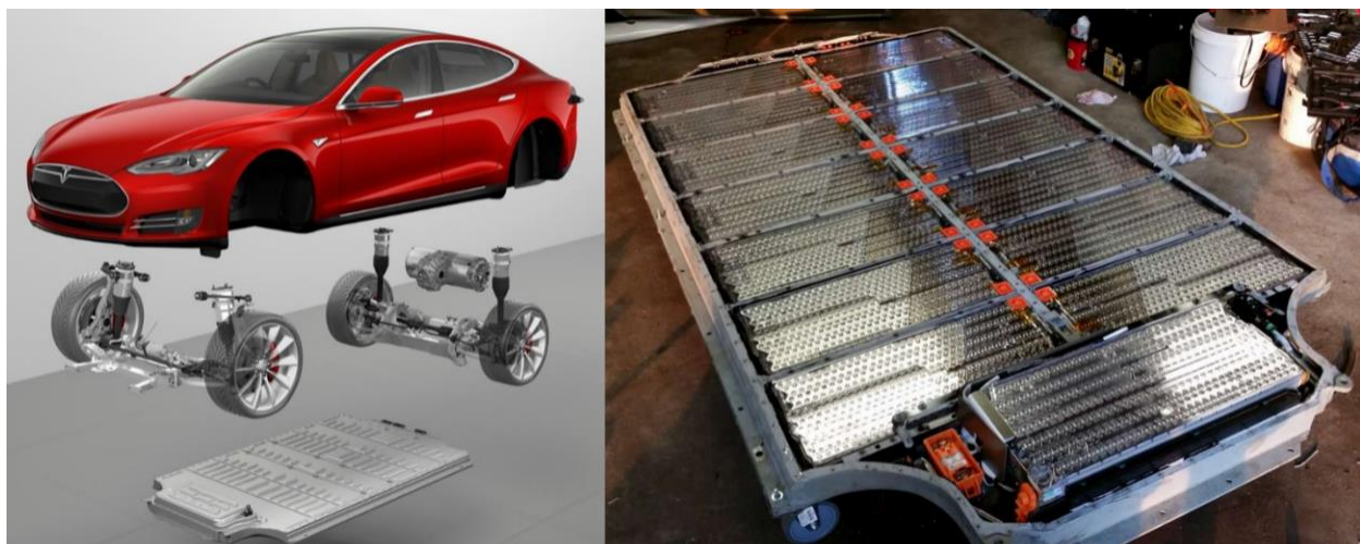
Figure 2-6: Left: Tesla Model S with 85 kWh LIB Pack (Bottom of Image, Source: Tesla.com) Right: Uncovered Pack [48]
