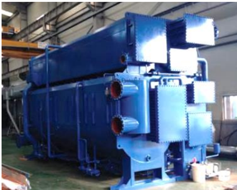
Figure 2-3: Maritime absorption chiller by Heinen & Hopman [43]
