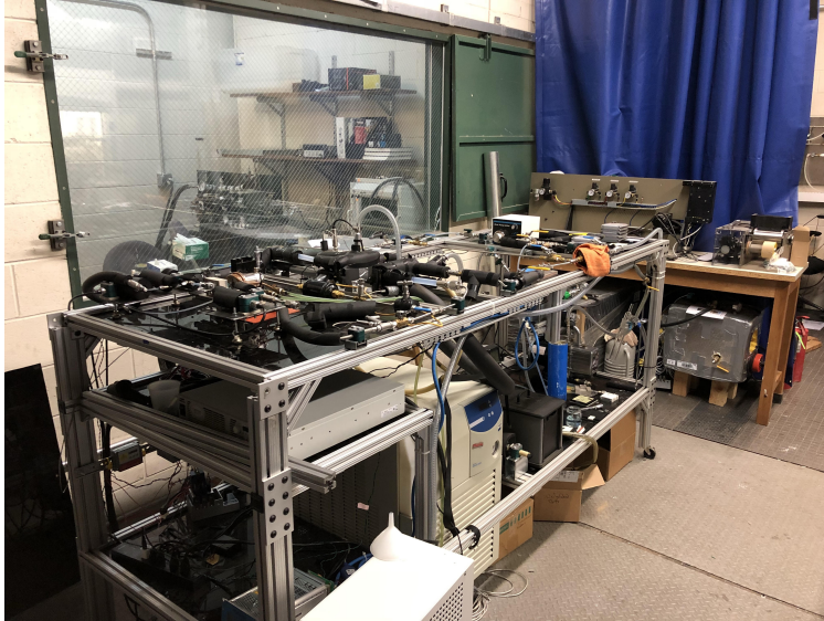
Figure 3.13: Image of custom designed heat transfer test facility. The test section interface is closest to the viewer and the gear pump lies at the back.
