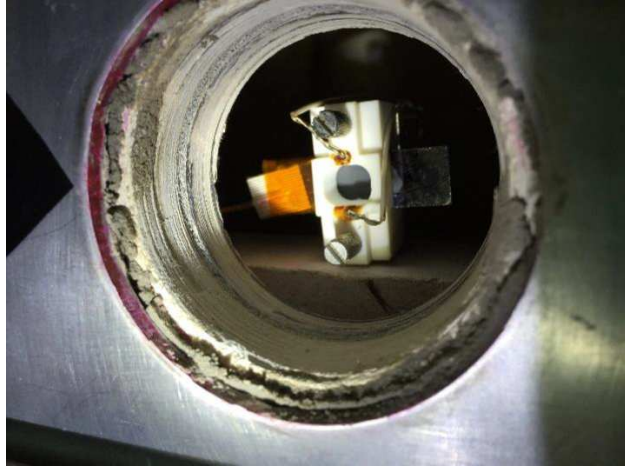
Figure B.3: Test section installed in electrical harness in calibration oven.
