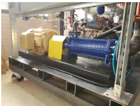
Figure 3-11 Power cycle pump and full speed performance curve (Adapted from [184])
