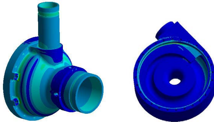
Figure B-15 Turbine (Left) and compressor (Right) finite element analysis strength assessment
