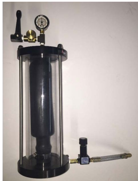
Figure 3-16: Accumulator removed from the test facility
