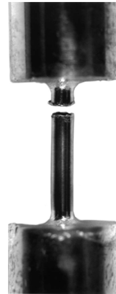
Figure 2-6: Image of two-phase burnout in a circular channel from Mudawar and Bowers [43]
