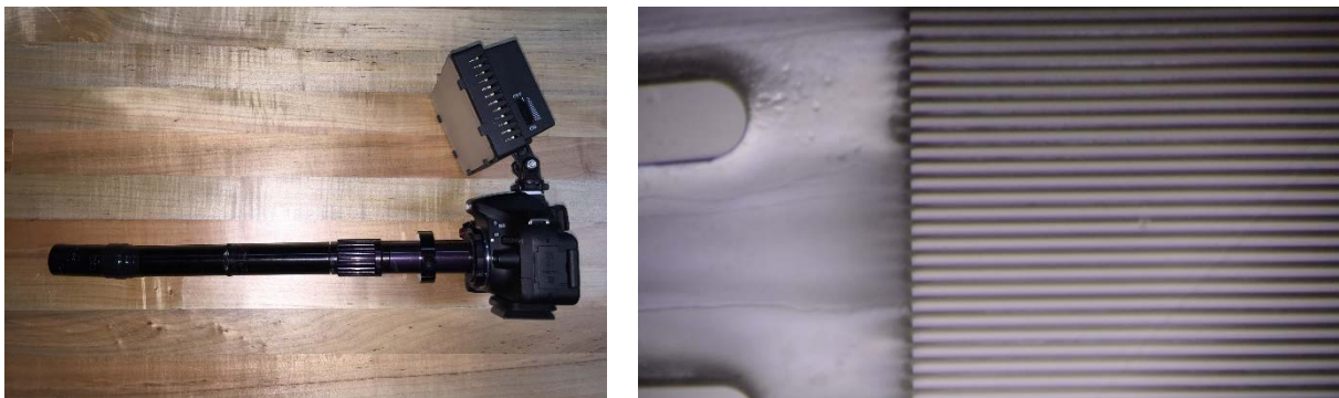
Figure 3-15: Left: Image of the camera with LED bar light and lens; Right: sample image
