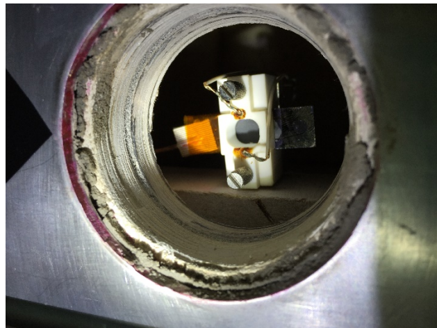
Figure B-19: Test section with thermocouple adhered to the silicon surface and place in heated cavity
